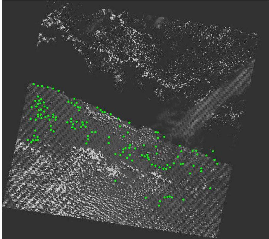
When the parameter for the ‘genchips’ algorithm was changed to 30x30 it produced about 709 points within the image. However, only 80 points registered successfully to produce a reliable solution.
