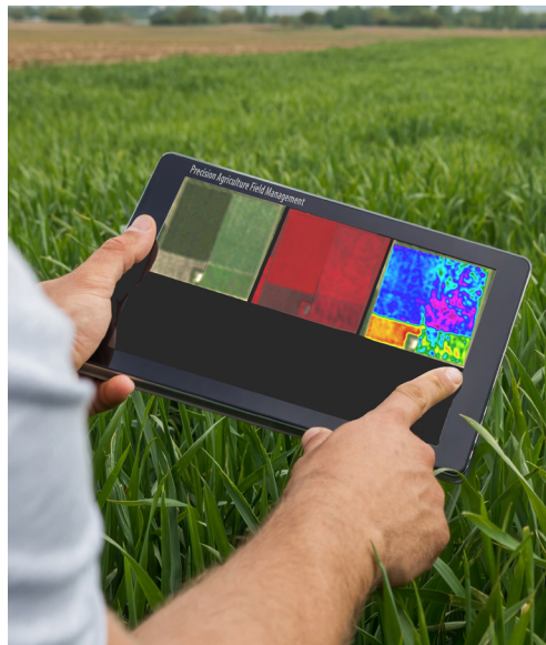
On the hand-held tablet above: Landsat 5 imagery collected July 13, 2005, of a sugar beet field, show a true color composite (left), color infrared (center), and near-infrared band (right) processed to show vegetation status related to nitrogen. In the (right) image, magenta indicates vigorous growth and high nitrogen; lighter green indicates low nitrogen and plants under stress. In the case of sugar beets, slight levels of stress are desired because stress maximizes development of sugar content. (From Gary Wagner, AWG Farms)
