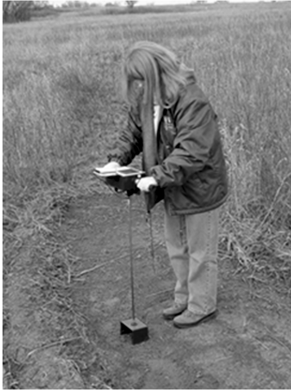
FIGURE 11.4 Picture of a cone penetrometer in use. The cone penetrometer shown is made by Rimik Pty. Ltd., Toowoomba, Queensland, Australia. Photograph courtesy of Dr Peggy S. Althoff, Kansas State University, Manhattan, Kansas.
