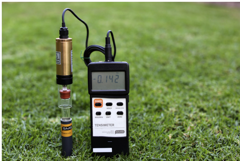
FIGURE 5.10 Photograph of the Tensimeter™ in field use. Courtesy of Soil Measurements Systems, Tucson, Arizona. (For color version of this figure, the reader is referred to the online version of this book.)
