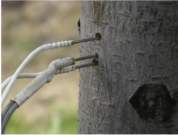
FIGURE 21.2 The heat-pulse method in use on an apple tree. Photograph courtesy of Steven R. Green, The New Zealand Institute for Plant and Food Research, Ltd., Palmerston North, New Zealand. (For color version of this figure, the reader is referred to the online version of this book.)
