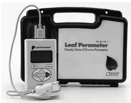
FIGURE 24.11 The steady-state diffusion porometer sold by Decagon Devices, Pullman, Washington. Photograph taken by Marsha K. Landis, Graphic Designer and Web Manager, Departments of Agronomy; Plant Pathology; and Horticulture, Forestry, and Recreation Resources, Kansas State University, Manhattan, Kansas. Used by permission of Marsha K. Landis.
